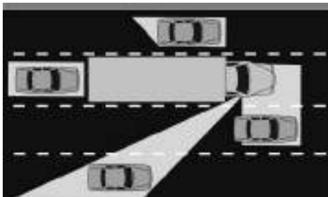
This diagram shows the various blind spots for a tractor-trailer
